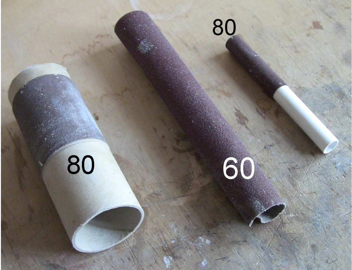
To facilitate the sanding operations I did made a couple of tools
