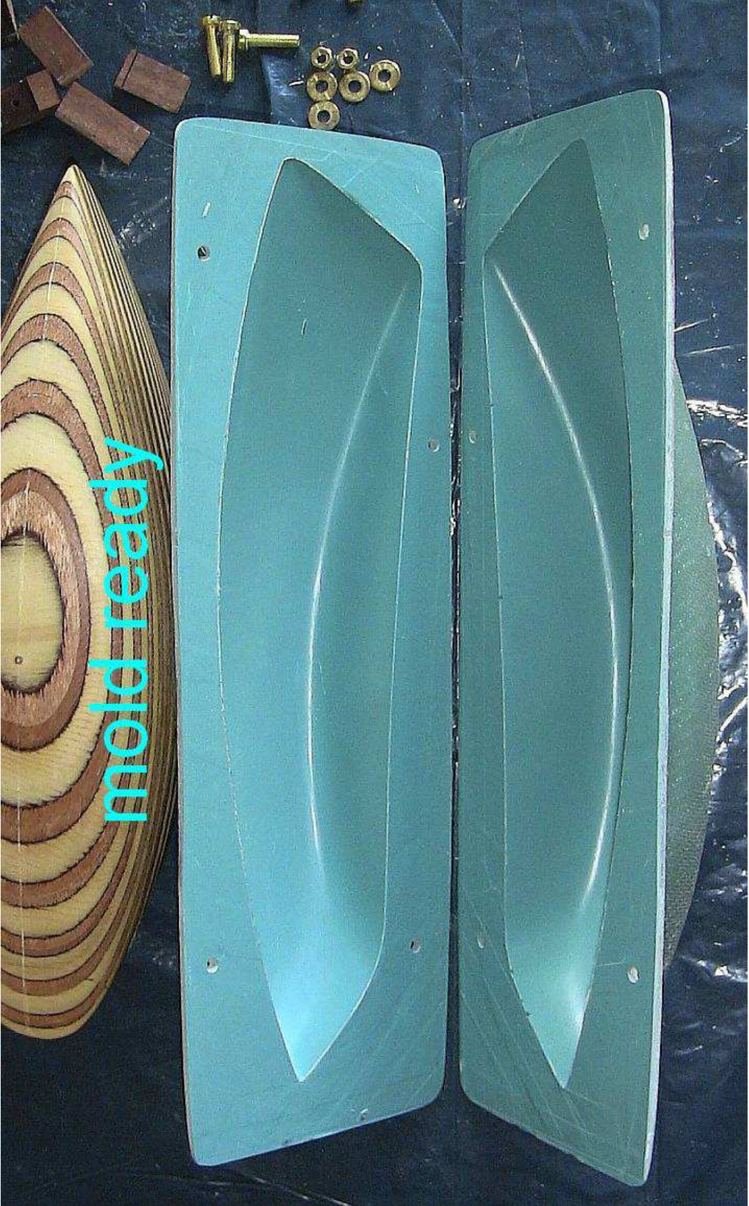
Clean view of the dual mold
