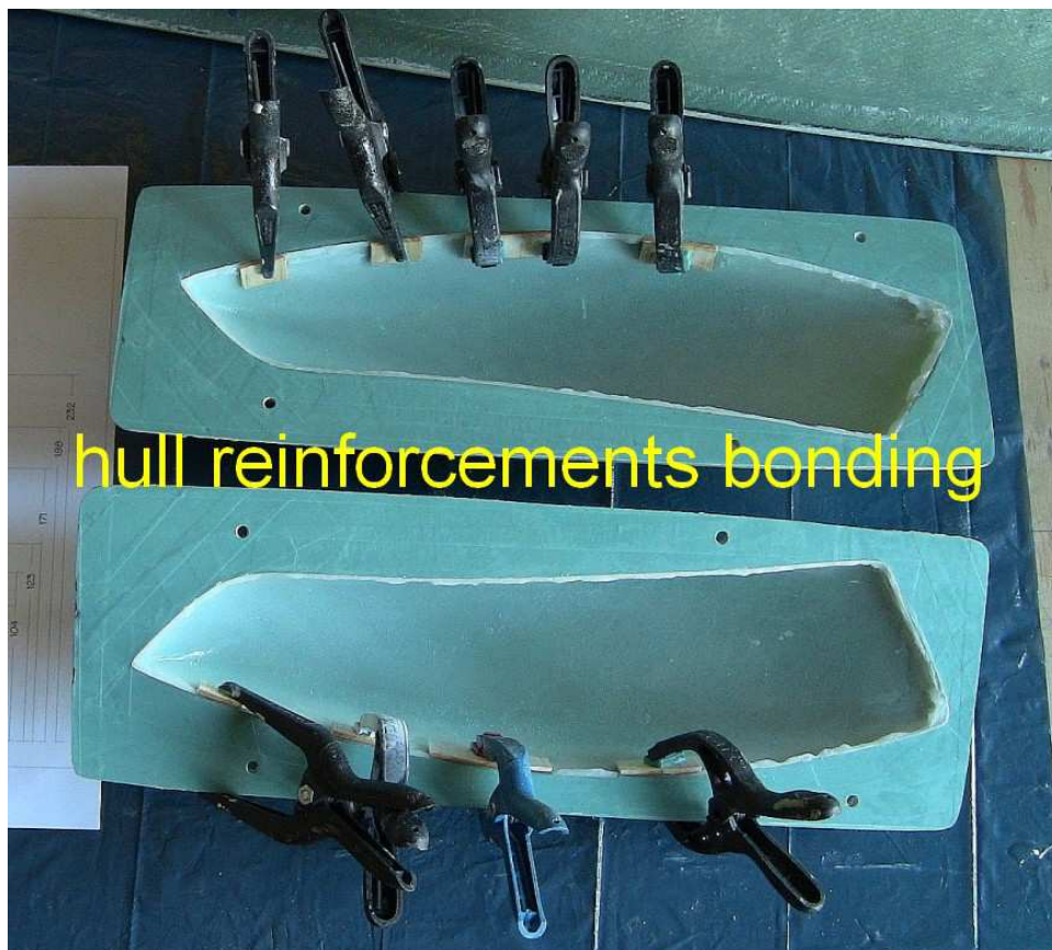
Inside wood reinforcements patches lamination
