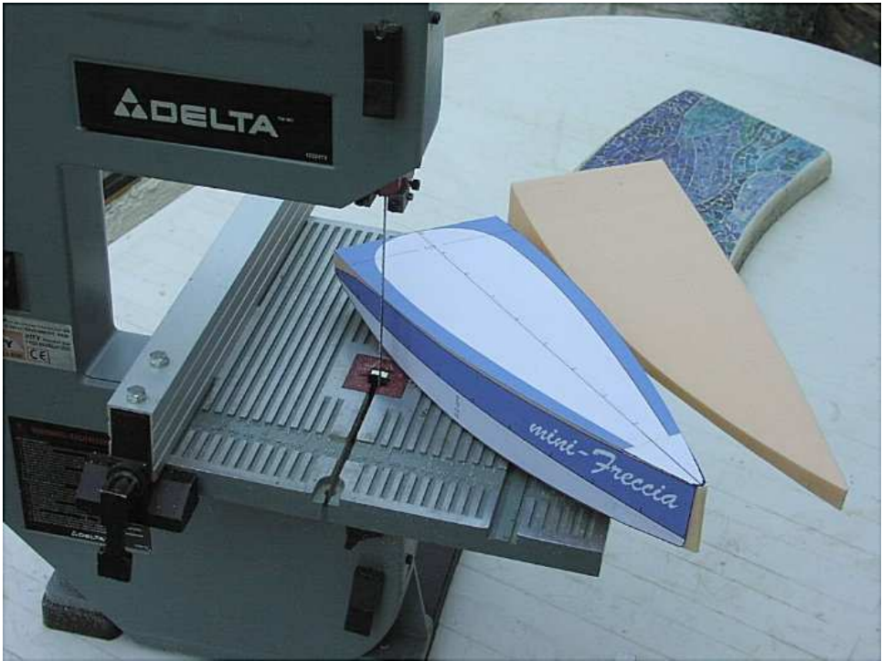
325mm basic block hull before smoothing
