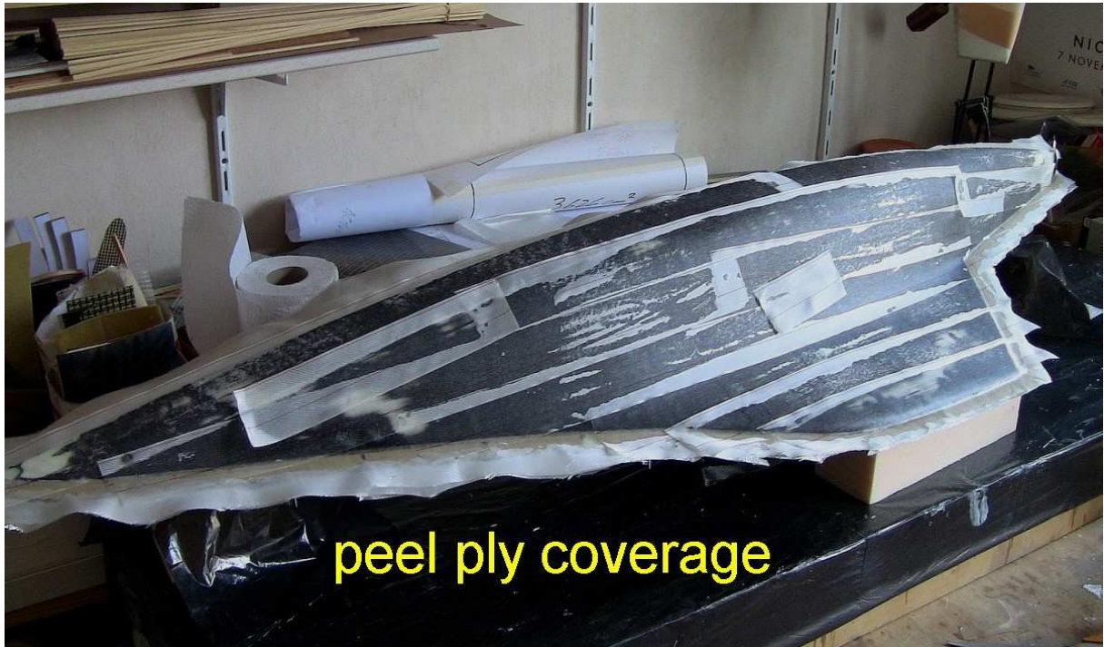
After lamination Peel ply tissue is used to absorb the Epoxy resin excess
