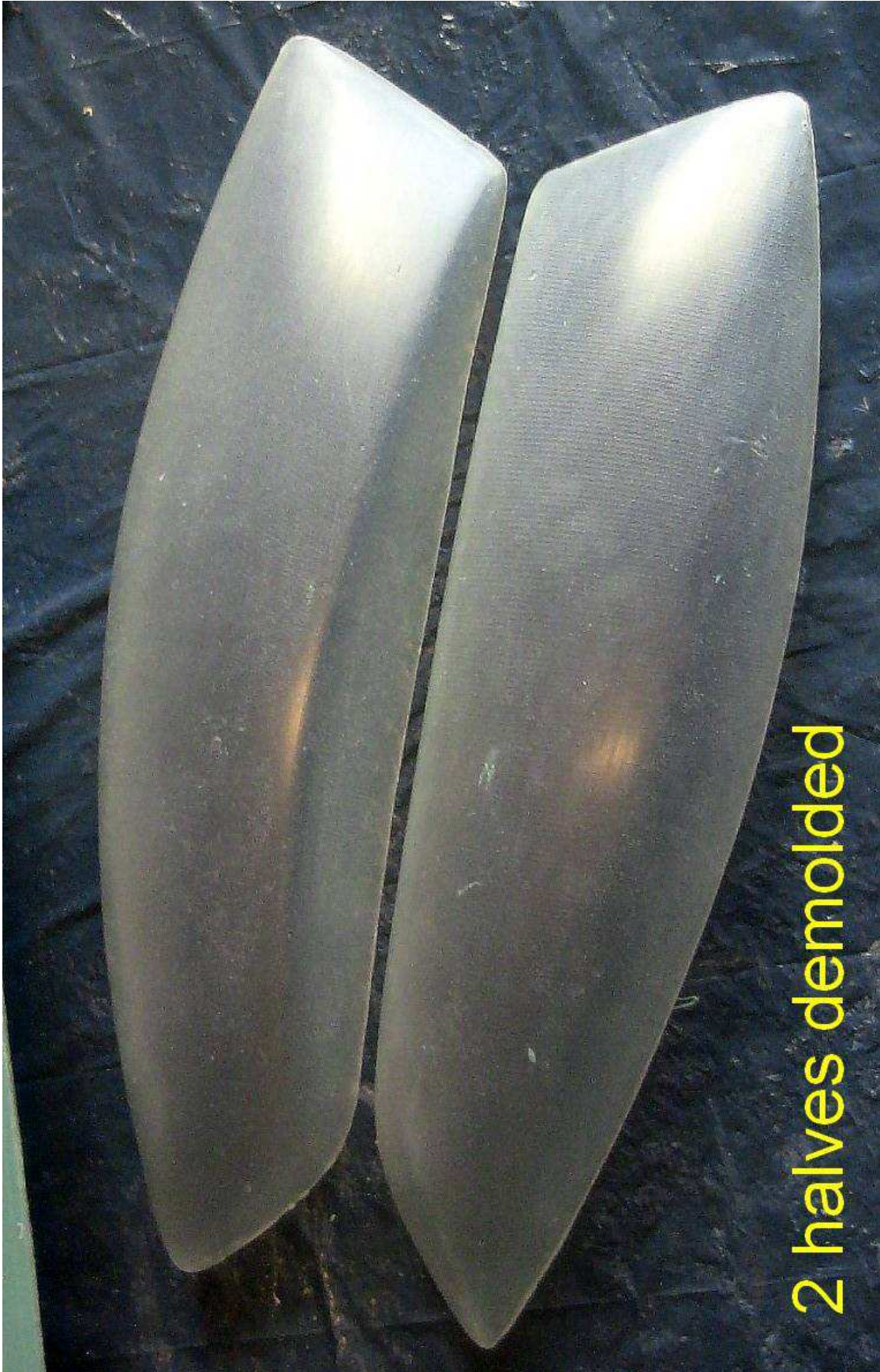
The two laminated hull halves
