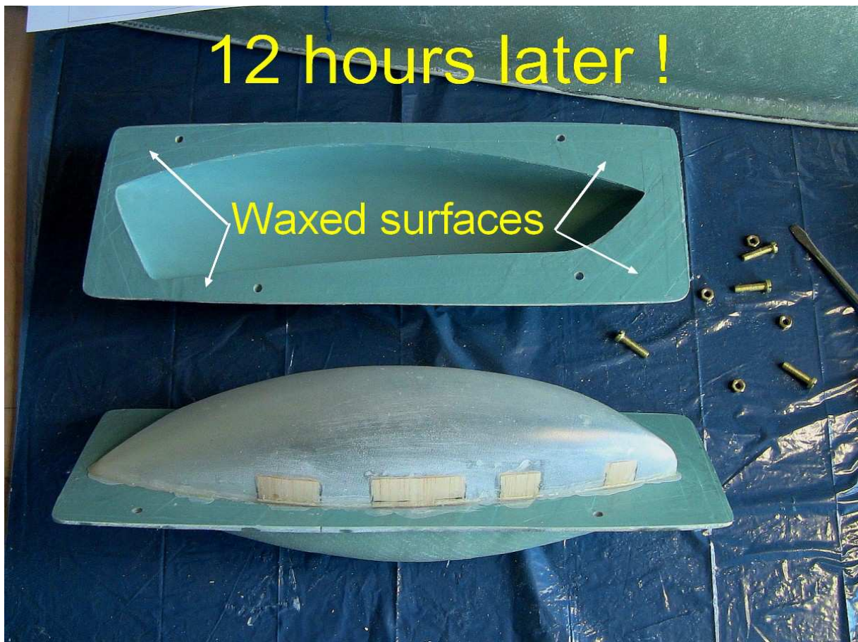
Epoxy-glass Hull out of the dual mold
