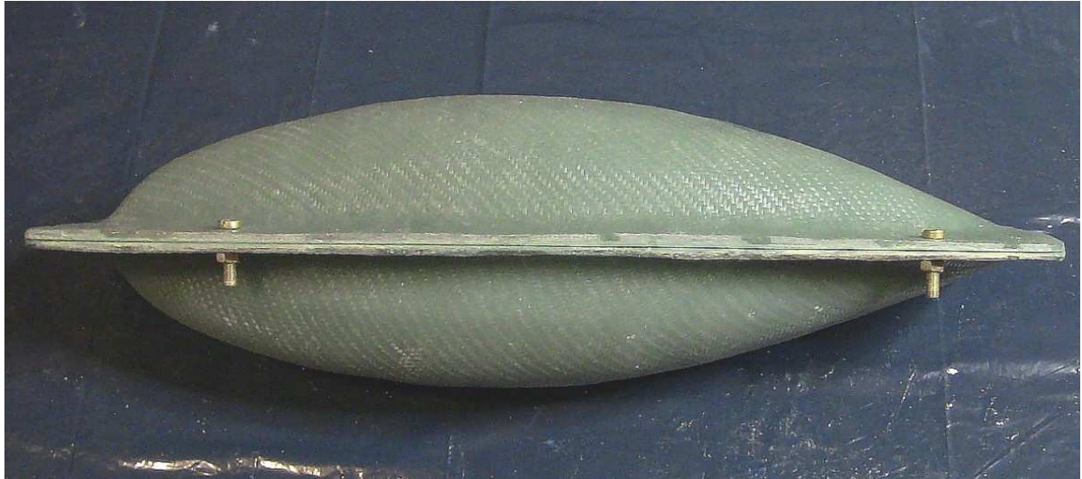
Mold closed after waxing waiting hull polymerization
