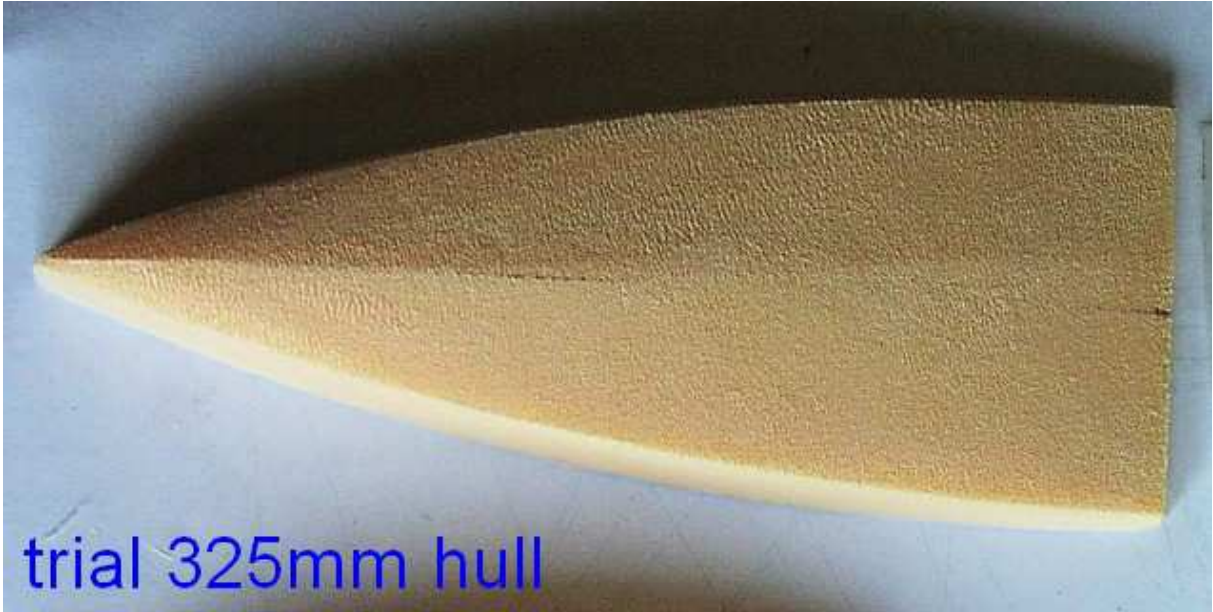
325mm basic block hull before smoothing
