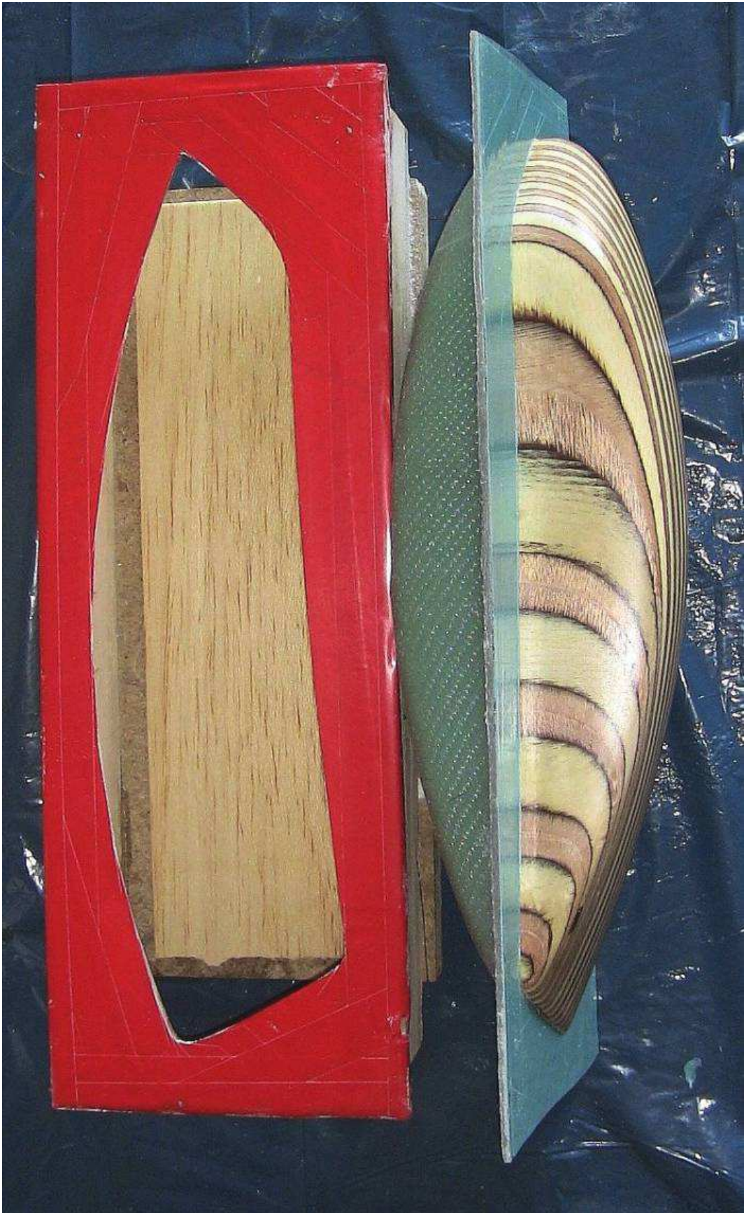
Half mold made and out of the jig
