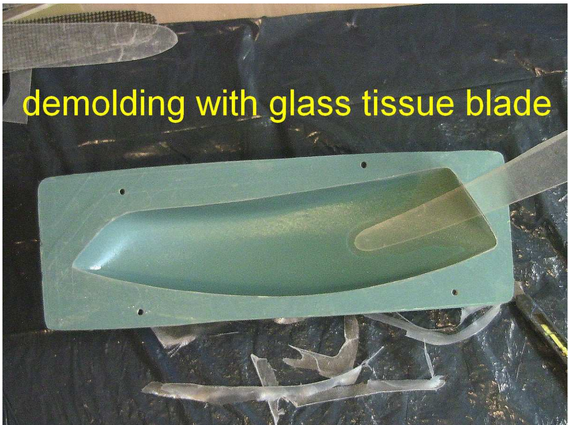
Removing excess of polymerized glass and extraction with laminated glass blade.
