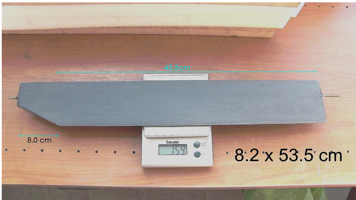
Second Fin plywood core trial
