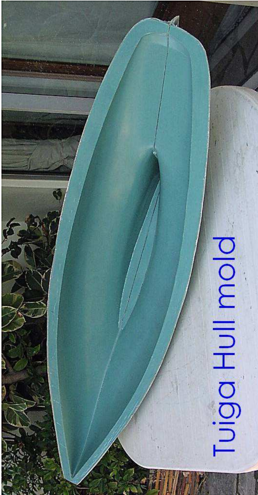
The two halves are joined with the use of bolts
