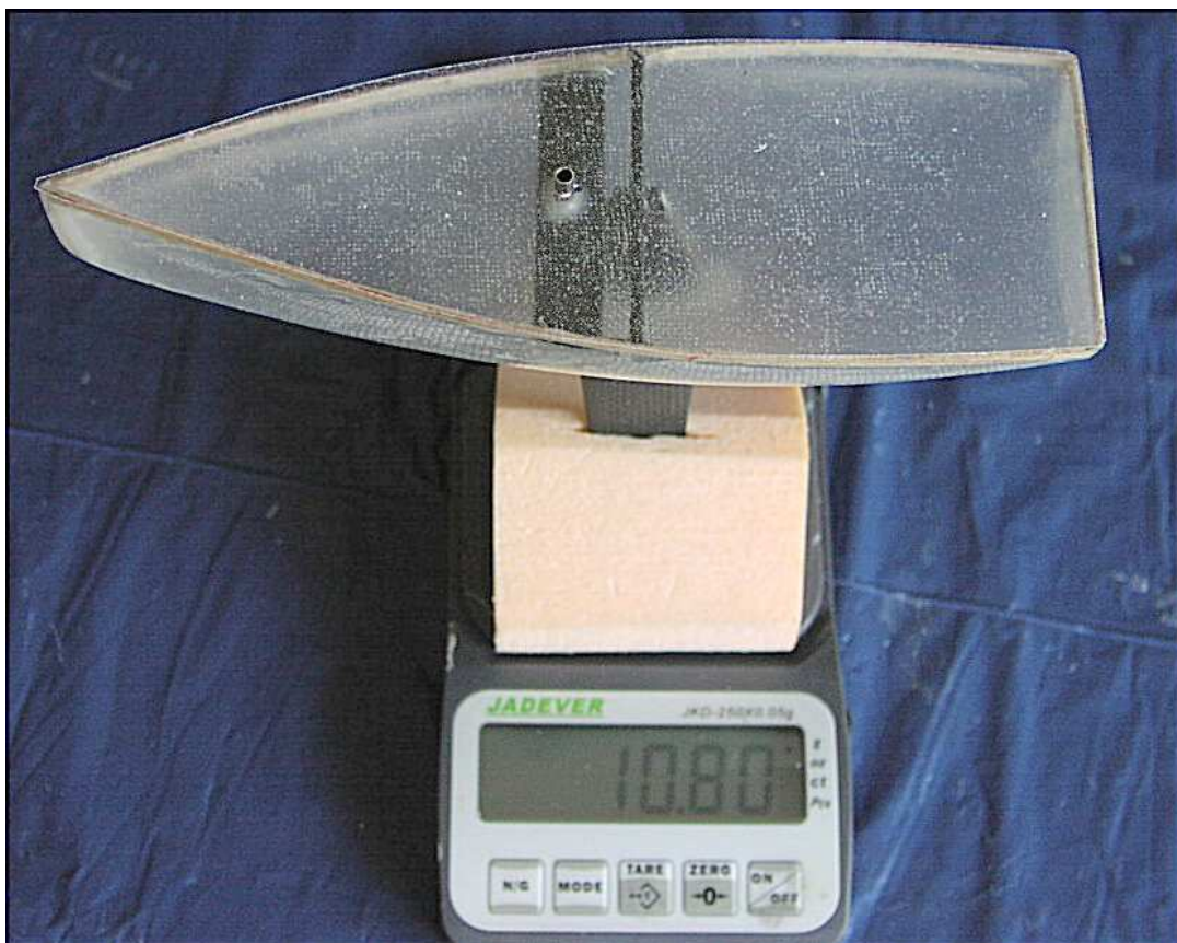
Hull and Deck weight 10.8 g including wood stringers
